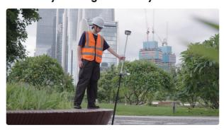
The VI0i supports the Tilt Survey of 60 degrees. We don't need to hold the survey pole upright when measured, which improves the efficiency of the measurement. When we meet some positions where we can't hold the pole upright, the Tilt Survey function will help you solve it easily.
